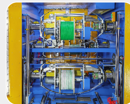
后面放线部分 Back-side back twist payoff
